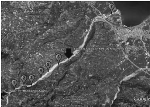
Fig. 4: Sampling map of Meganitis stream. The paddles show the sample stations. The black arrow shows a zone of aggregate quarry. The black concave arrow shows the joining of a tributary with the main channel.
