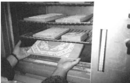
Figure 7. Drying process of glazed tiles samples
