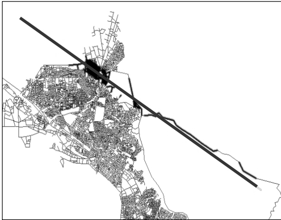
Figure 7. The extra (to those depicted in Fig. 5) inaccessible road links due to destruction of the road axes by rupture zone of Asvestochori2 (thick black line) are depicted in black colour (scenario 3, case 3).
